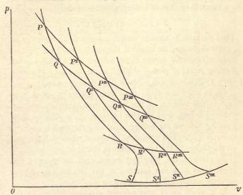
equal to one another. Thus the absolute temperatures in any two isothermals PP' and QQ' are to one another as the complete areas PP'Q'R'SSRQ and QQ'R'S'SR. The determination of the ratio of these areas, when PP' and QQ' belong to any two definite temperatures, such as those of water boiling, and of ice melting, under one atmosphere of pressure, is a matter entirely for experiment. (How such
